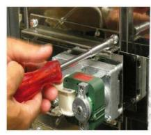
Remove the engine and grease shield
