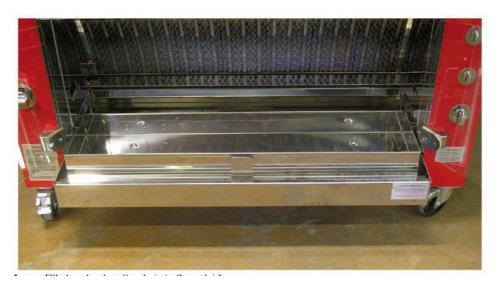
To drain the fat, slide the drip tray out of the unit and lift the drip tray slightly to angle towards the drain.
