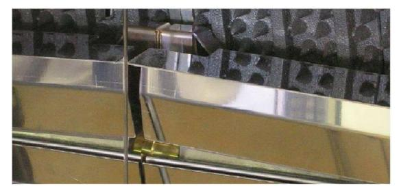
To replace the burner cover, position the lower T part between the burner and the burner support
