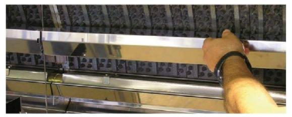
Lift the burner covers, being careful not to scratch them against the back of the unit Remove the burner cover
