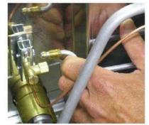
· Remove the feeding tube gas pilot.
