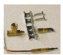
Remove the two screws from the pilot and thermocouple retaining flange Remove the pilot and thermocouple
