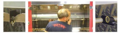
Now insert the right hand side into the hex shaped fitting which is attached to the motor
