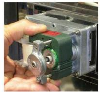
Remove the 2 screws of the coil using a Phillips screwdriver. Remove the assembly
