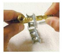
Attach the new pilot and align the holes
