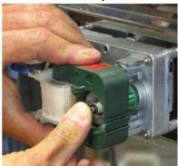
Remove the coil Remove the Rotor
