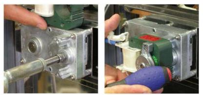
Using a grease gun, squeeze grease into the hole of the rotor axis two or three times Replace the rotor, coil, assembly and screws.
