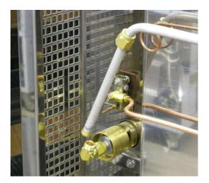
•Dismantle the 90 °elbow / nozzle holder and nozzle.
