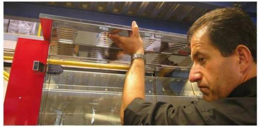
Slide the deflector into the slide brackets on the top of the rotisserie...
