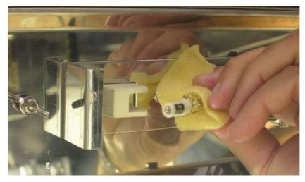
Turn off the power to the unit Open the glass doors Loosen the two thumb screws on the globe cover Lift off the globe cover Remove the halogen globe and replace it with a new one being careful to not touch the globe with your fingers Replace the globe cover Tighten the two thumb screws Close the units doors Reconnect the power
