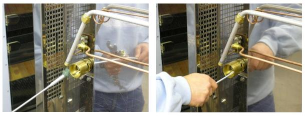
•Refit the elbow at 90 °/ nozzle holder, nozzle checking the settings outlined in the manual. •Tighten the nut of the 90 °elbow / nozzle holder, nozzle and check for any leaks.
