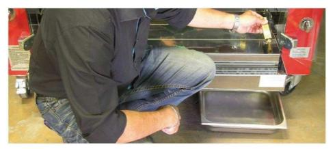
Place a small tray underneath the drain and remove the drain plug to empty the fat Replace the drain plug after cleaning the tray and place back into the rotisserie.
