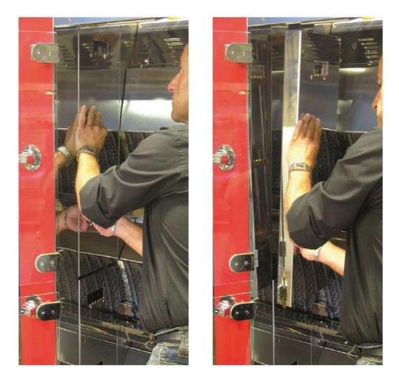
3.8 REMOVAL AND FITTING OF DOUBLE INNER PANELS
