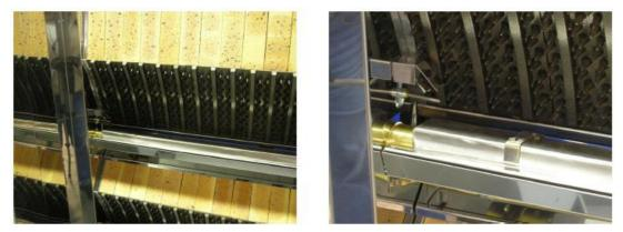
Close the stop valve of the gas supply and vacuum the remaining gas the drain the burners
