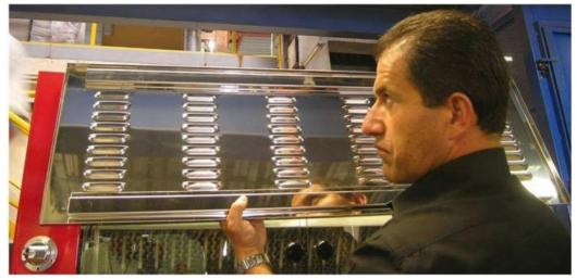
Place the deflector so that the two braces are directed upward with the open vents facing the rear.
