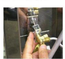
· Remove all pilot / thermocouple.
