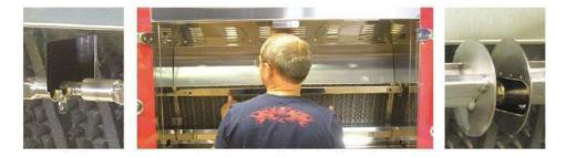
Lastly, put the left cylindrical end of the spindle into the groove in the wall panel
