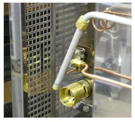
•Use a cloth soaked with rubbing alcohol on the end of a long rod to clean the inside of the burner
