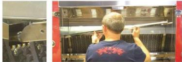
Insert the end of the spindle into the bearing located on the left panel
