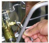
Unscrew the hollow screw connecting the gas supply tube to the pilot with a wrench 10.
