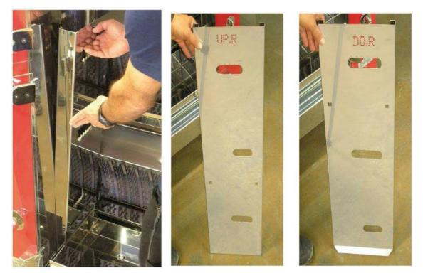
Proceed in the same way for the double bottom wall and those located on the other side The double walled upper right is punched with the letters UP.R.
