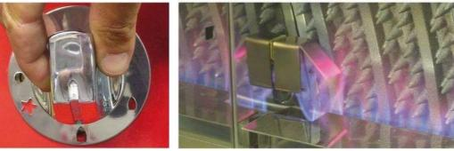
· To light the burners turn to the position heat maximum.
