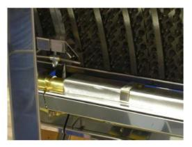
Remove the burner cover Loosen the two M4 screws and remove Clean the grill with a cloth soaked in rubbing alcohol
