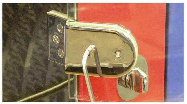
Unscrew the two countersunk screws from the front of each hinge with an allen key or BTR 4mm hex Remove the front hinges, two joints front and rear Put a new gasket on the back of each hinge Mount the new glass being careful that the sticker on it is positioned towards the inside of the rotisserie. Put another new gasket on the front of each hinge Replace the front hinges and tighten screws with countersunk heads Peel off the label of the glass Replace the door handle
