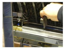
Refit all spark gas and tighten the two M4 screws Replace the burner cover and check the burner
